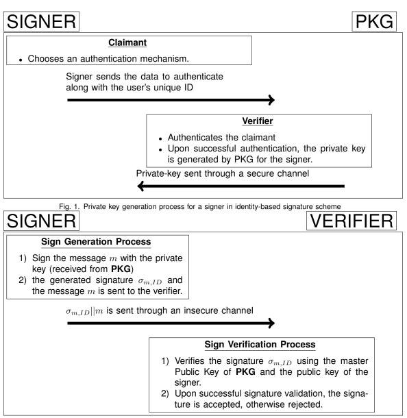
Fig. 2. Signing and verification of signature in IBS
